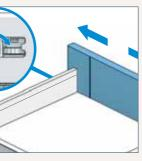
To adjust the drawer front horizontally, rotate the screw clockwise/ anti-clockwise.
