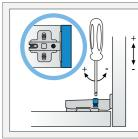
Side adjustment The side adjustment is made by
